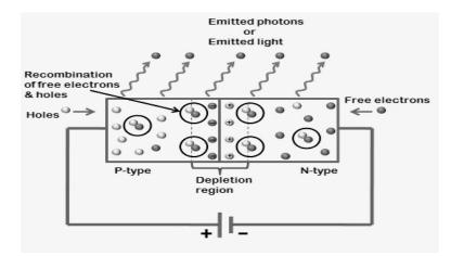
Figure 2-3: LED Lamp Circuit
