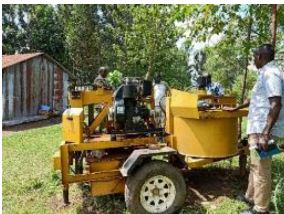
Plate 4.2: Hydraform ISSB Machine and Makiga ISSB Machine
