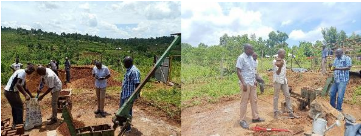
Plate 5.7: ISSB Production using Makiga Manual Press Machine at Kakrao in Migori.
