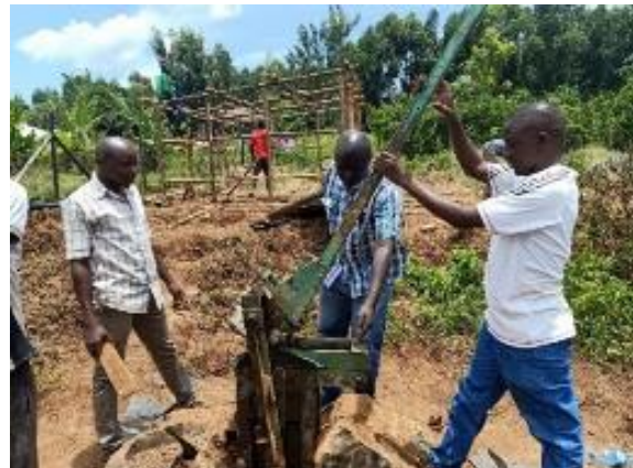
Plate 4.2: Hydraform ISSB Machine and Makiga ISSB Machine
