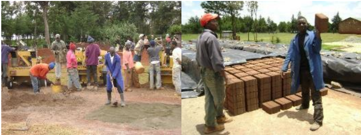
Plate 2.1 ISSB Material Preparation and Production
