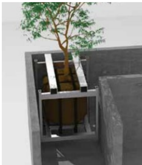
Figure 2.21: Bosco Verticale's redundant bind Source: (Giacomello, 2015)
