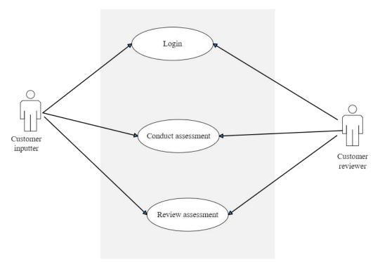
Figure 7: Customer inputter and reviewer use case diagram
