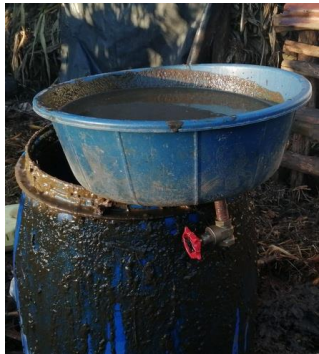
Figure 3.22: Substrate loading gate valve set up.
