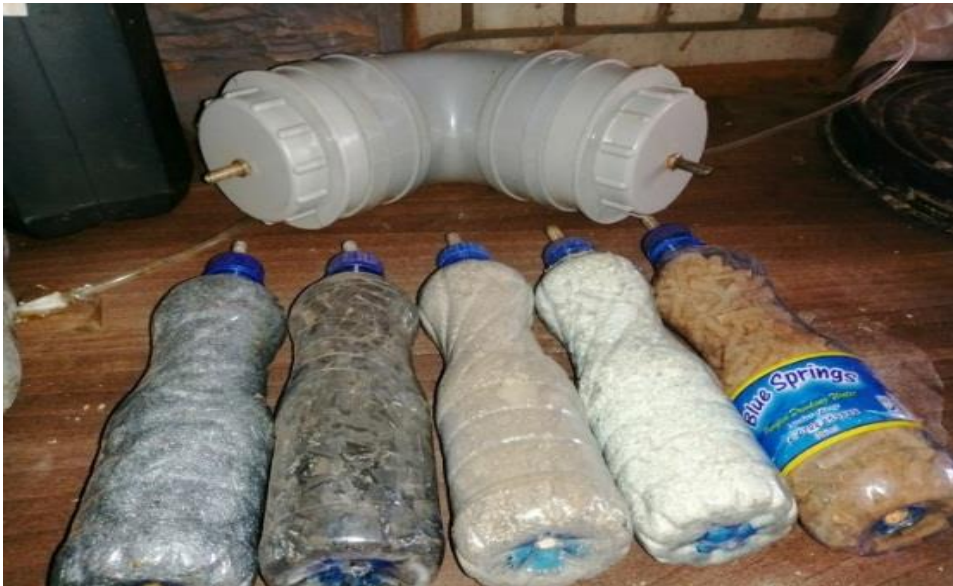
Figure 3.16: The biogas upgrading cartridges; rubber tires, natural zeolite rocks, commercial desulphurizer, maize cobs and steel wire.
