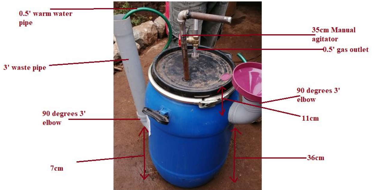
Figure 5.1: Schematic of the 60 L digester.
