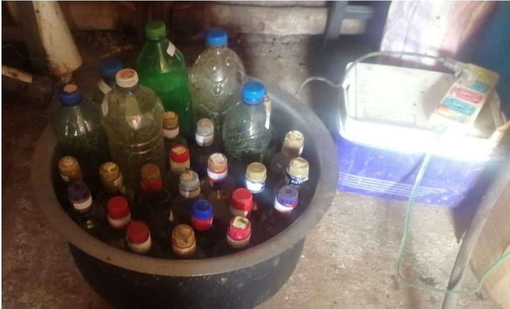
Figure 3.12: A setup of fruits and vegetable market wastes pretreatment process The same procedure was repeated using twenty fruits and vegetable markets wastes using NaOH in place of HCl to compare acid hydrolysis to alkaline pretreatment.
