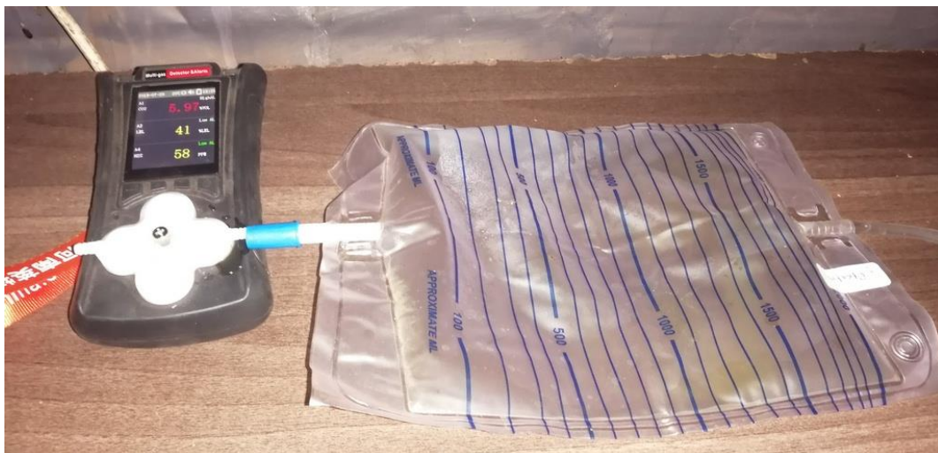
Figure 3.11: Biogas analyzer measuring biogas quality from potato waste
