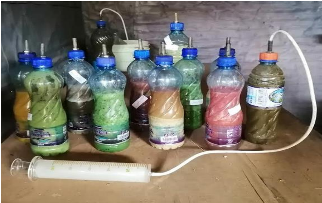
Figure 3.6 : Biogas production set up at psychrophilic conditions.
