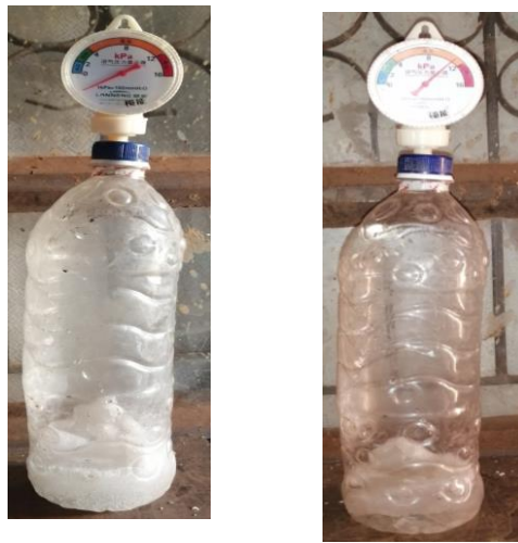
Figure 3.2: Pressure test setup for 1 liter bottle.
