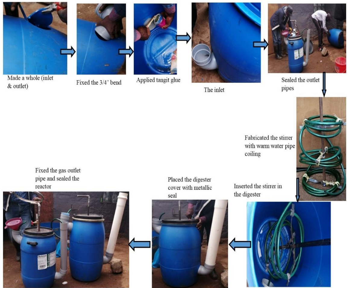
Figure 5.5: Fabrication of plastic drum digester steps
