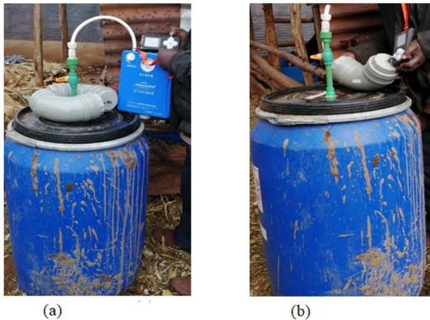
Figure 3.36: Pilot-scale biogas upgrade setup (a) using a desulphurizer (b) using zeolite
