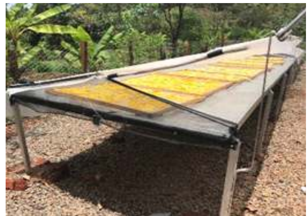
Mango fruit slices drying in a tunnel solar dryer at the Karurumo Aggregation Centre
