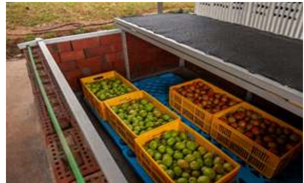
Zero Energy Brick Cooler: One of the low-cost cold storage technologies at the Demo unit
