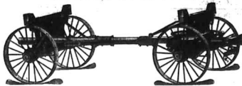
"ELECTRIC" ALL-STEEL WAGONS, with Wheels Mounted on long Improved Ball-bearing Axles, making them very light in draft. Supplied in capacities from 400 to 16000 pounds capacity. Prices on application.
