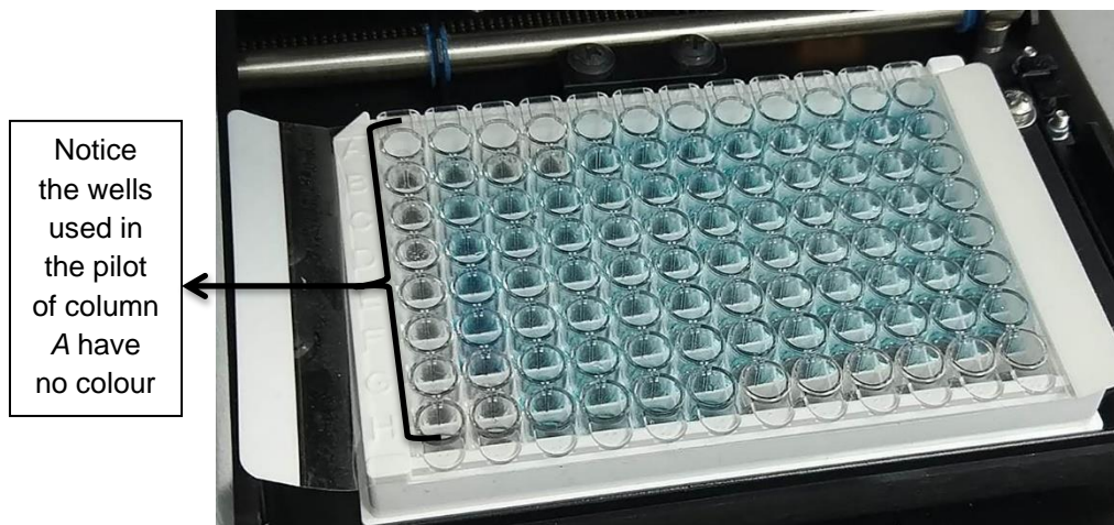
Figure 8: Plate being placed into a dark chamber for incubation
