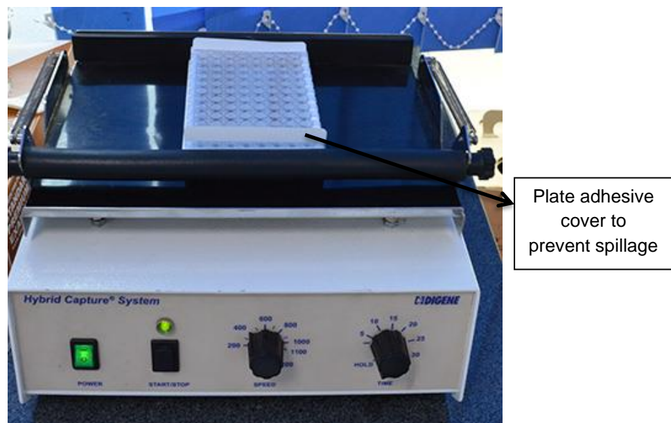
Figure 6: Plate rotator, securely holds plate, with variable RPM and timer
