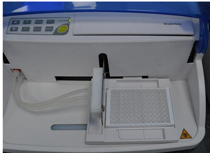
Figure 7: Plate washer calibrated for six, 300 \mu L cycles
