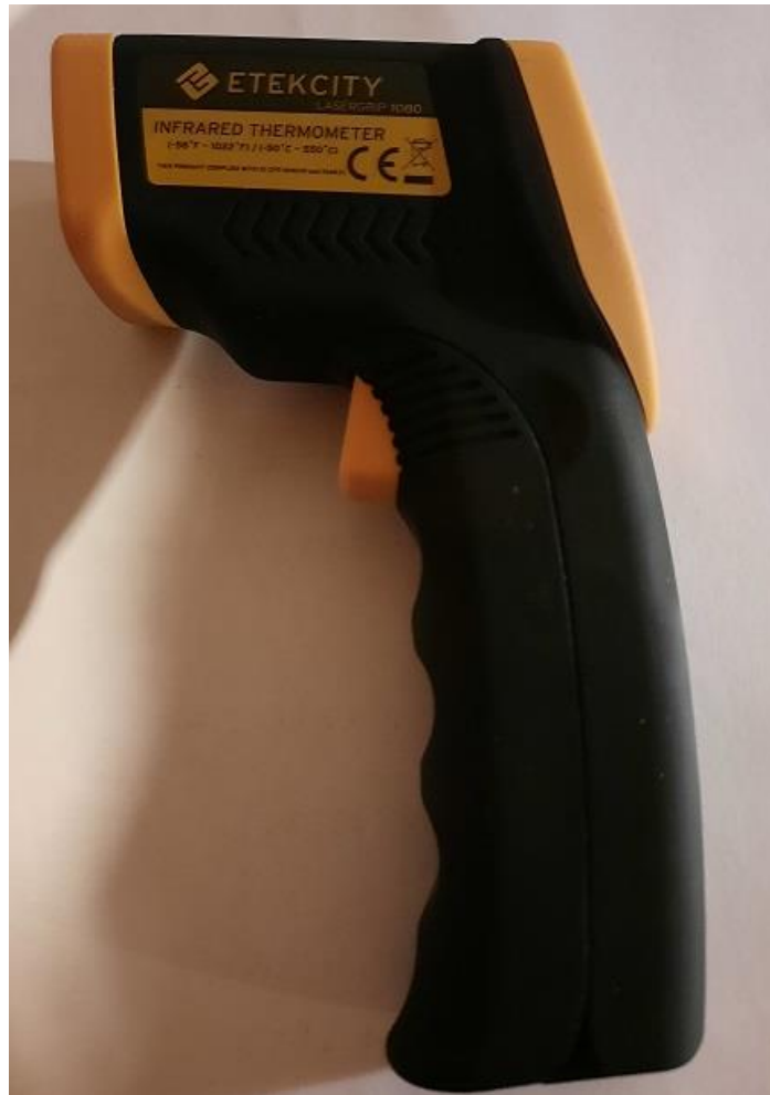
Image 7: Infrared thermometer designed for inanimate object temperature monitoring, used to determine temperature suitability of temporary storage box for samples during data collection period.
