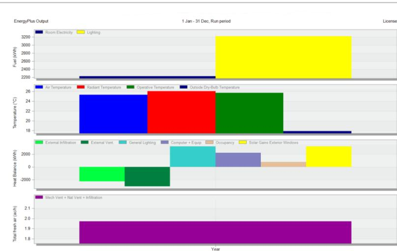
Figure 4-11: Classroom U-1 energy simulation graph as existing with shading device
