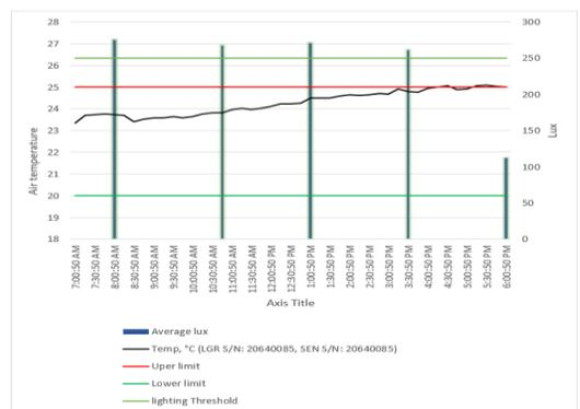
Indoor air temperature records the least time of overheating due to delayed heat transfer (less than one hour) compared to aluminium, wherein indoor air temperature increases shortly after exposure of the shading to the sun and reduces drastically on non-exposure.
