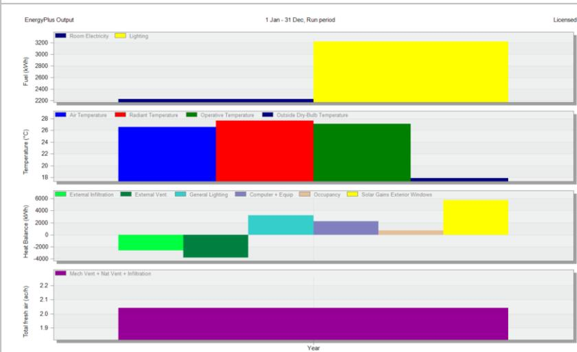
Figure 4-12: Classroom U-1 energy simulation graph without shading
