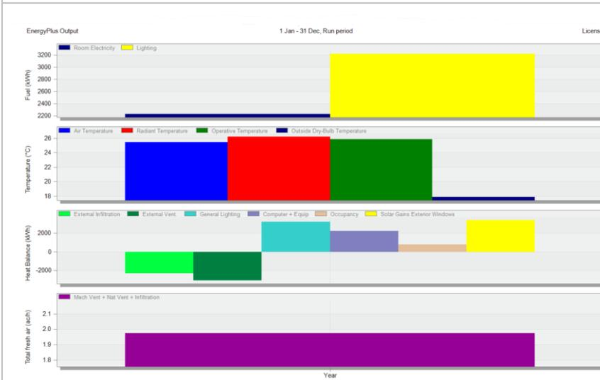
Figure 4-15: Classroom U-2 energy simulation graph as existing with shading device
