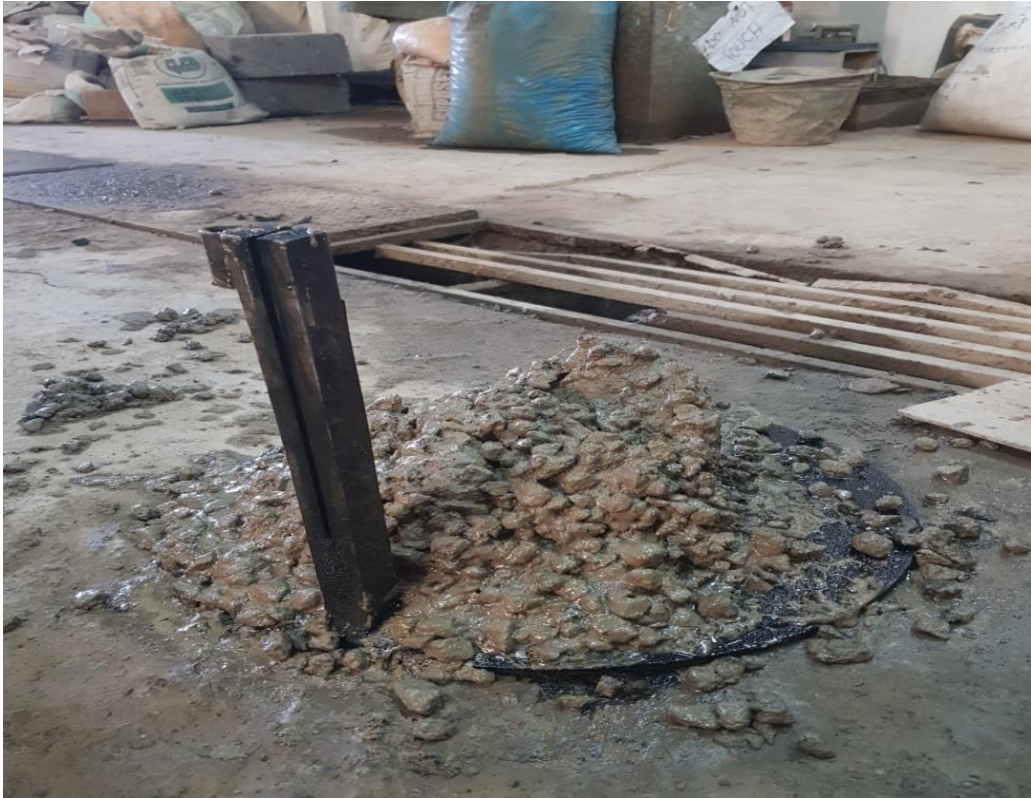
Plate 4.1: Collapse slump of a concrete mix (Source: Author)
