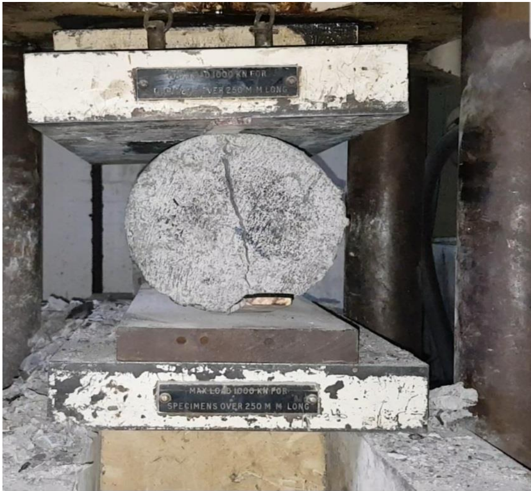
Plate 4.6: Conventional concrete specimen tested for splitting tensile strength. (Source: Author)
