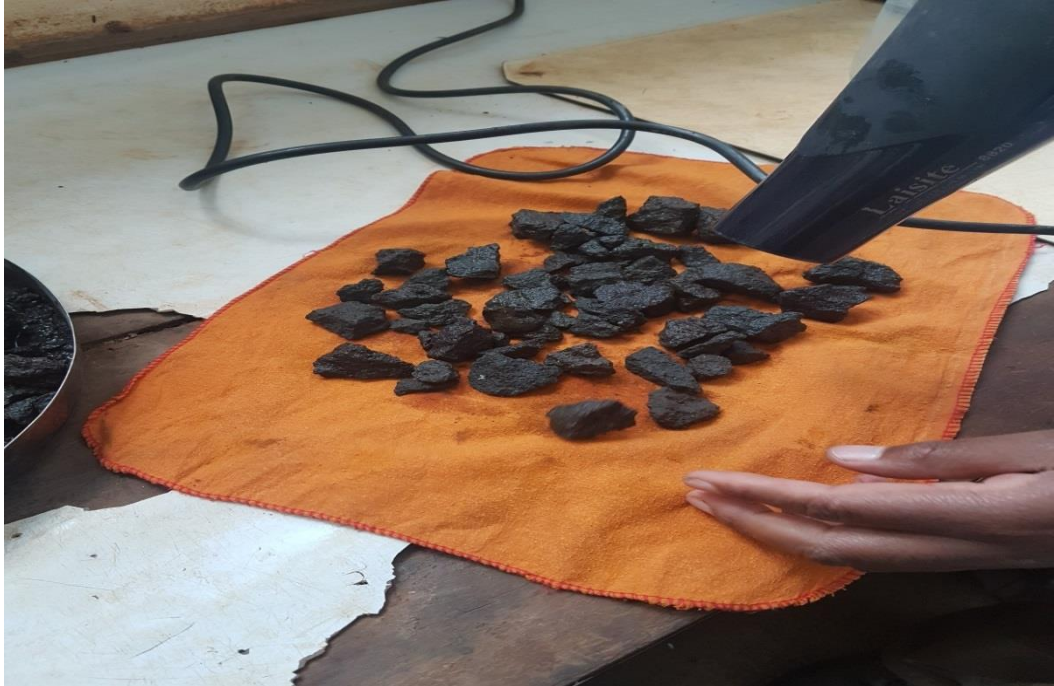
Plate 3.6: Sample of SSD tuff aggregate sample. (Source: Author)
