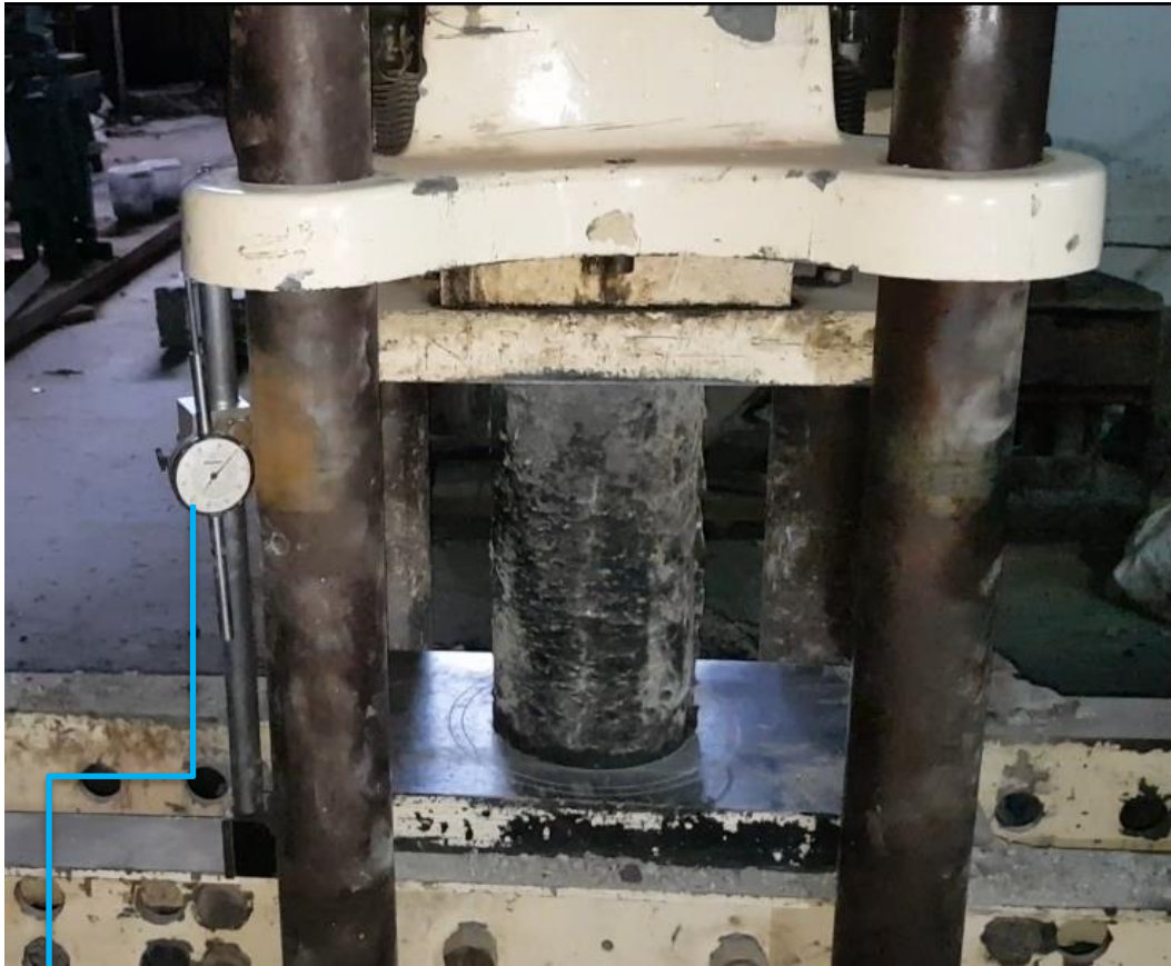
Plate 3.10: Cylindrical specimen being tested for elastic modulus.
