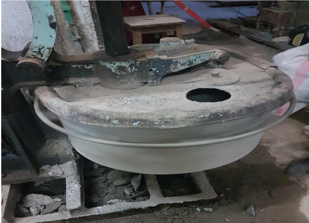
Plate 3.7: Mixing of concrete materials in a rotating mixer in the lab. (Source: Author)
