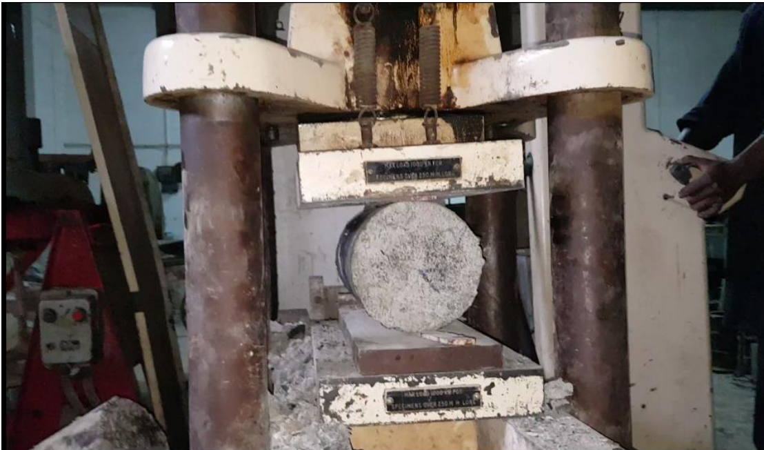
Plate 3.9: Cylindrical specimen being tested for splitting tensile strength.
