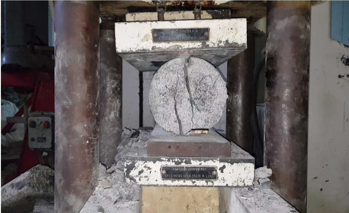
Plate 4.5: Cylindrical tuff concrete specimen tested for splitting tensile strength (Source: Author)
