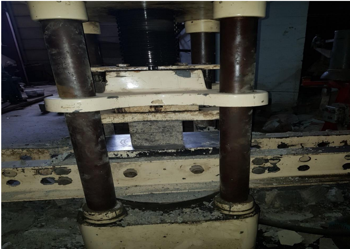
Plate 3.8: Cube specimen being tested for compressive strength. (Source: Author)
