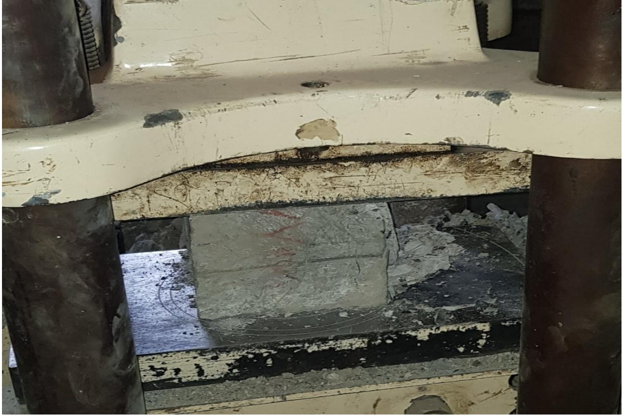
Plate 4.4: Failure mode of normal -weight concrete cube specimen
