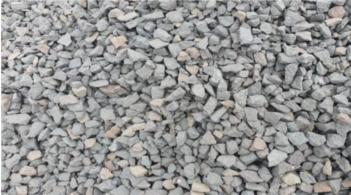
Plate 3.3: A sample of tuff aggregates from Bahati quarry. (Source: Author)
