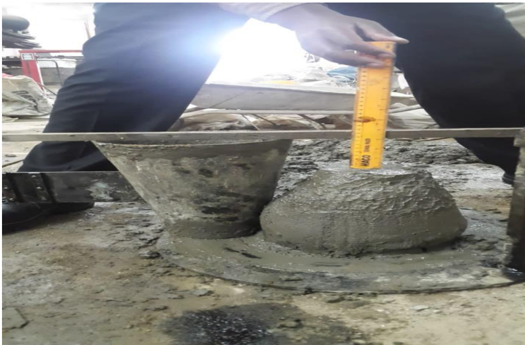
Plate 4.2: True slump of a concrete mix (Source: Author)
