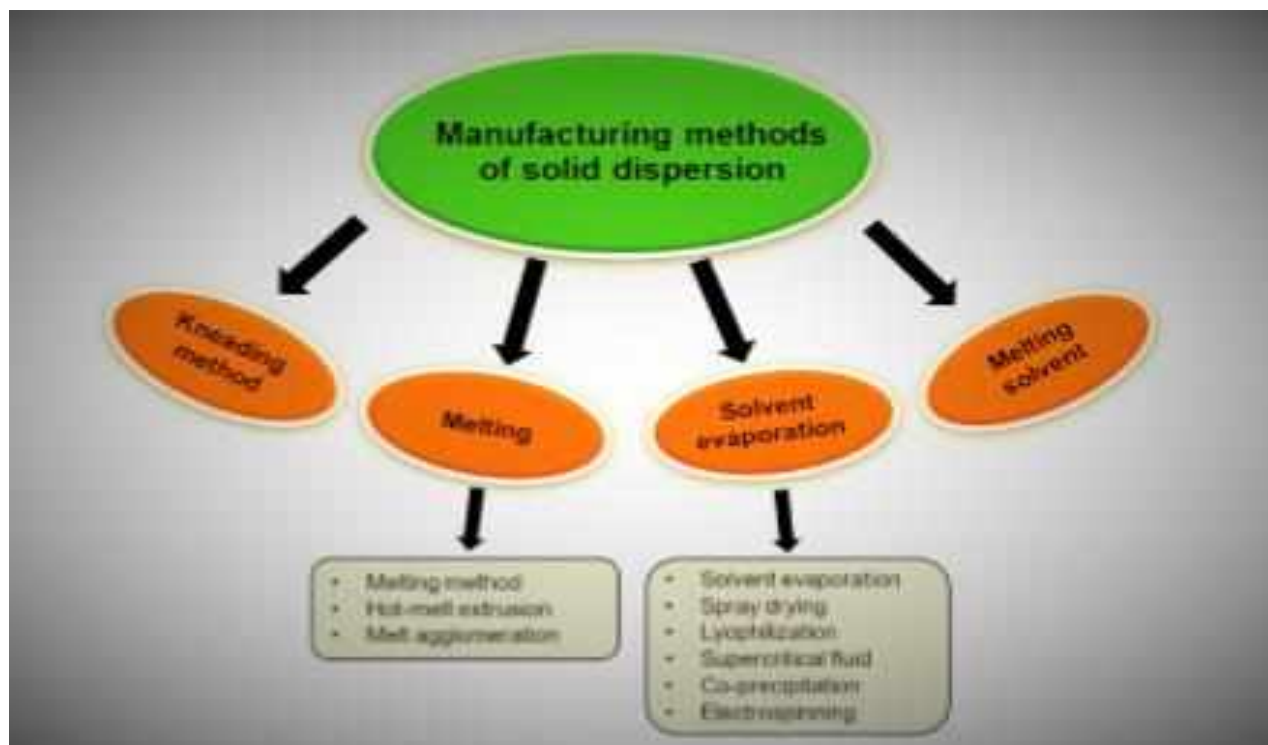
Figure 2.3: Manufacturing methods of solid dispersions (Tran et al., 2019).
