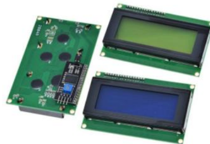
LCD2004+I2C 2004 20x4 2004A Blue/Green screen HD44780 Character LCD /w IIC/I2C Serial Interface Adapter Module For Arduino
