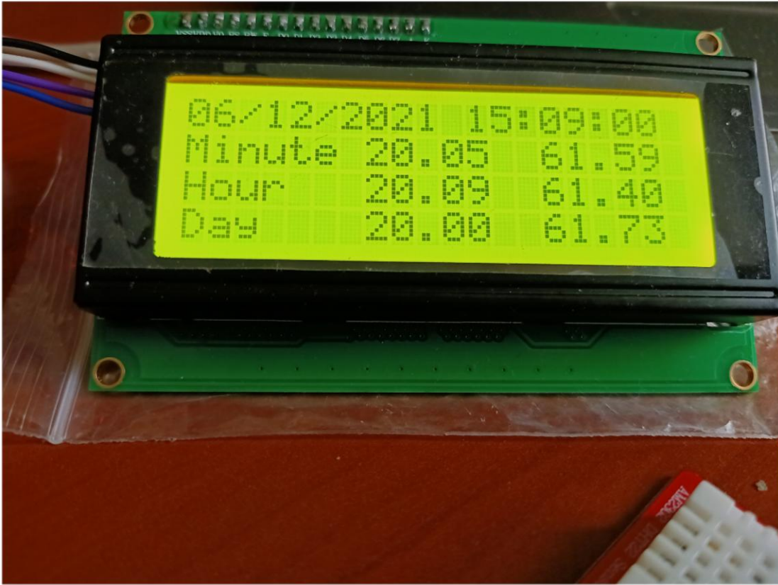
Figure 12 the LCD display, showing the instantaneous temperature and humidity readings and also cumulative readings for the hour and day.
