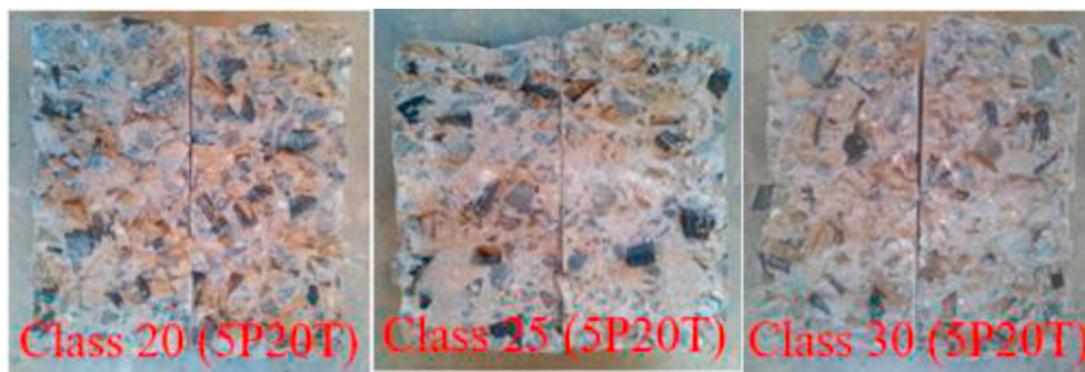
Figure 16. Rubber distributions in cylinder specimens broken after 28 days curing period.
