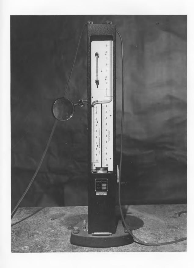
Figure 8. Density bottle. Mercury fills the void space up to the level indicated by the pointer
