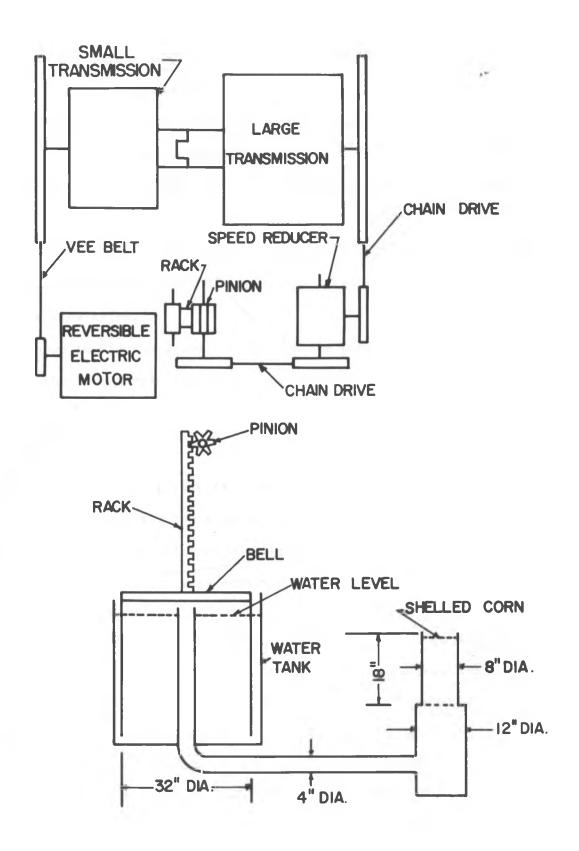
bottom of the tank with open end extending above the water surface to serve as an air outlet (and inlet) and a bell driven up and down at known speed by a driving mechanism.
