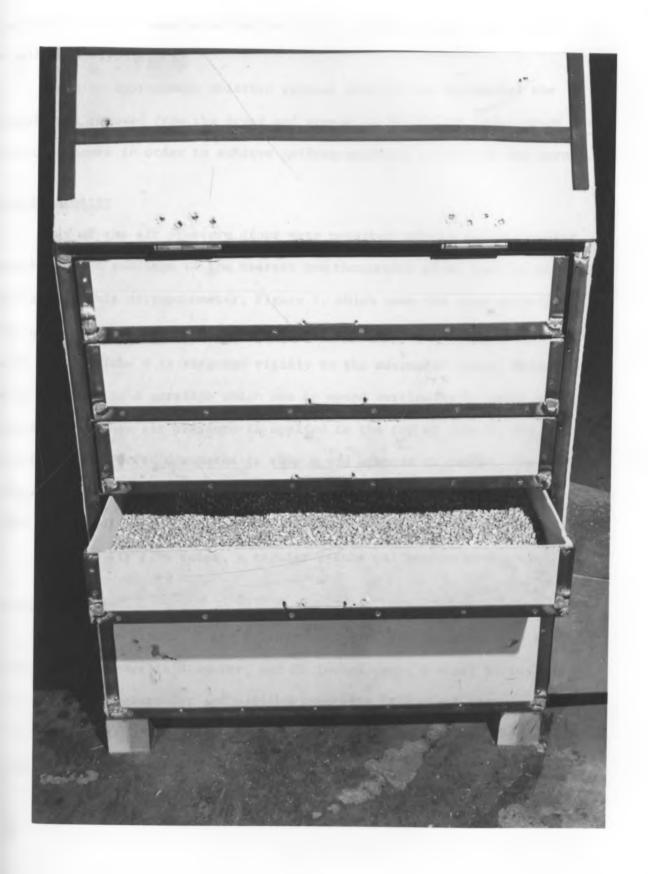
possible to dry 4 samples of shelled corn to different moisture levels simultaneously.
