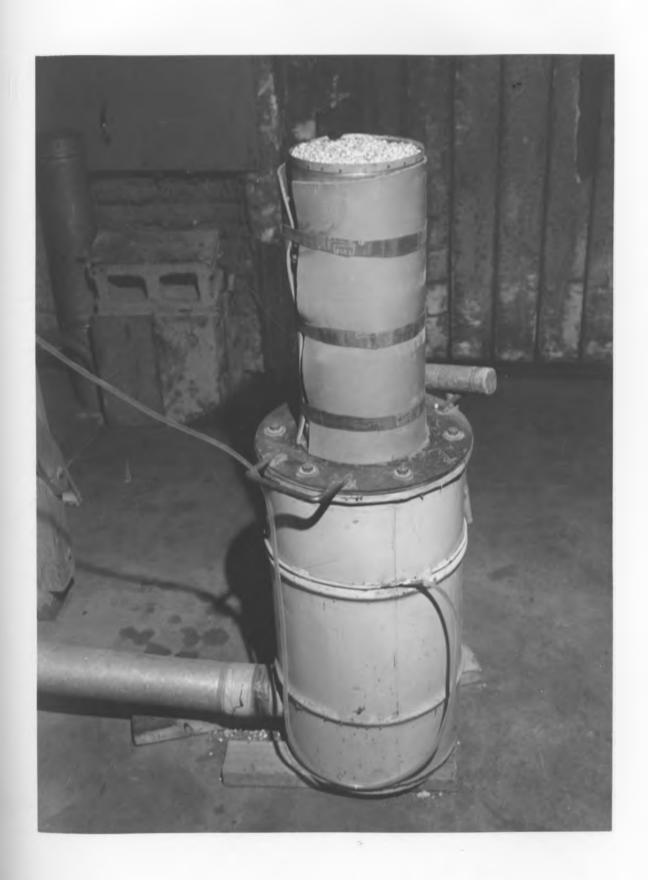
Figure 5. Dryer assembly showing dryer cabinet, intersection air duct, electric heater unit, and the temperature control
