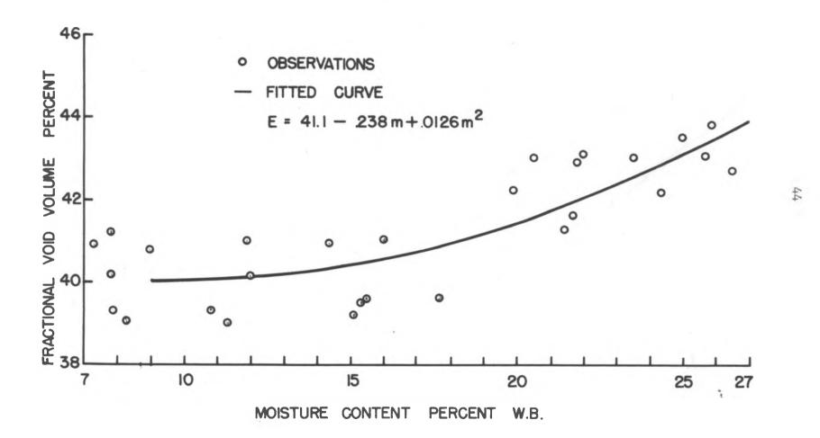
Figure 11. A plot of fractional void volume vs. moisture content for packed filled shelled corn
