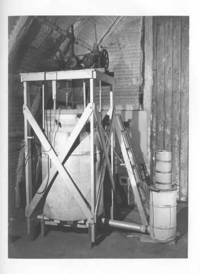
Figure 4. Plenum and test bin of Shedd's apparatus
