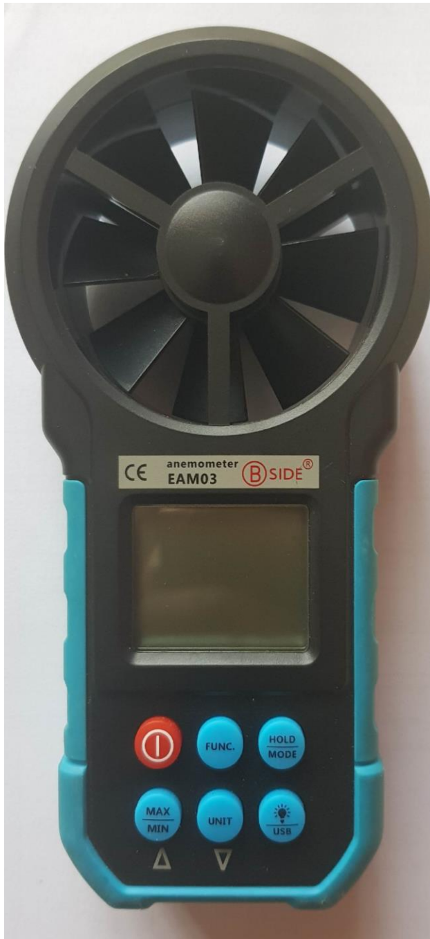
Figure 6.1: Rotating vane anemometer that was used during the field study Source: Author
