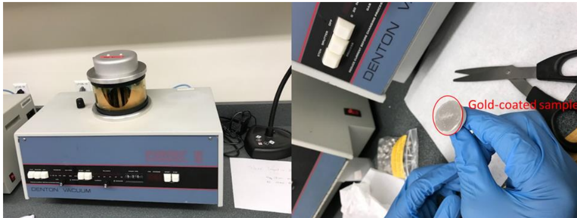
Figure 4.2: The setup of the Denton Vacuum sputter coater at 100 milliTorr used for coating the samples.
