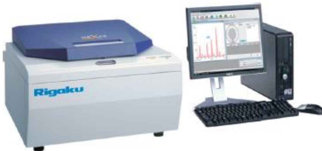
Figure 4.1: The Energy Dispersive X-Ray Fluorescence Spectrometer used in elemental analysis of diatomaceous earth and the binder
