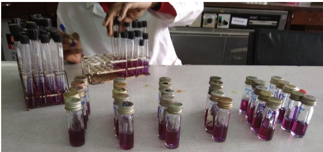
Figure 4.3: The pure double and single strength MacConkey Broth Purple w/ BCP solution filtered by the fabricated membranes
