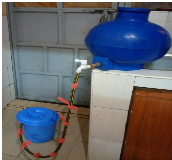
Figure 4.10: The setup used to filter contaminated water across the 0.8 T magnetic field
