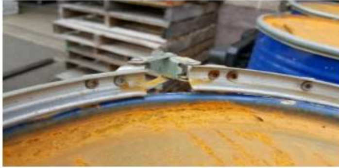
Figure 2.4: Red Rust (Albanycountyfasteners.com, 2021)
