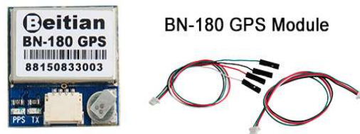
Figure 4.2: Beitian BN-180 GPS Module. Amazon (2021).
