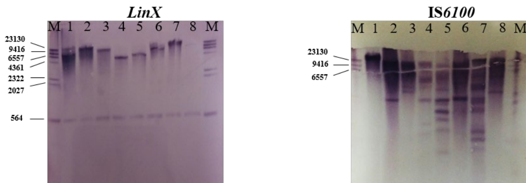
Figure 9. Southern blot hybridization of genomic DNA of Sphingobium sp. S6 showing nitrocellulose membrane hybridized with LinX and IS6100 DNA probes. M: DIG-labeled Mol. wt marker, LinX –IS6100 Lanes 1 to 8, genomic DNA digested with Bam HI, Eco RI, Eco RV, Hind III, Pst I, Sac I, Sal I, and Xho I, respectively.
