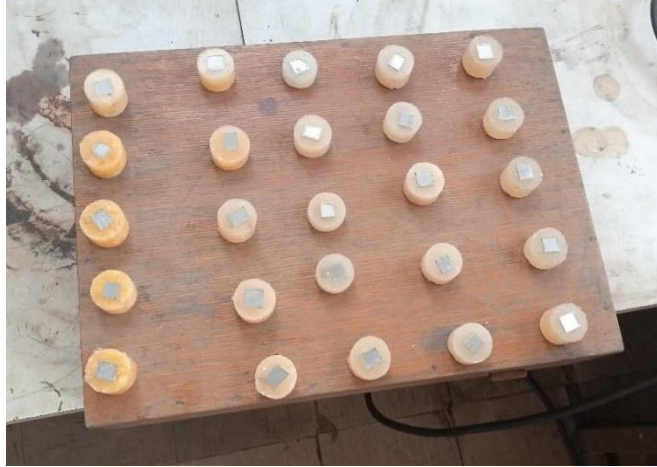
Figure 3.21: Mounted specimens for micrography and hardness test.
