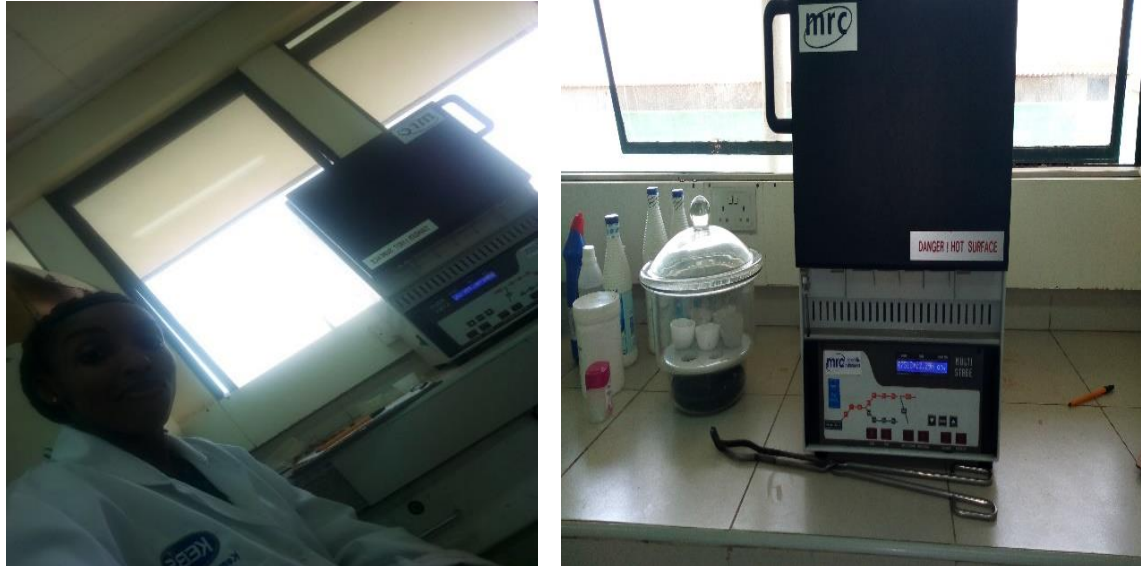
Figure 3.6: Thermal enhancement using the muffle furnace in Kenya Bureau of Standards (KEBS).
