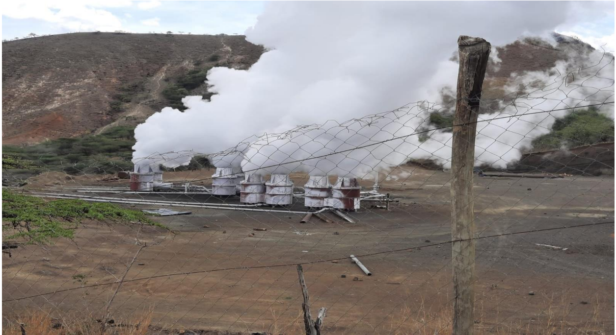
Plate 4. 6: Discharging well with Hydrogen Sulfide
