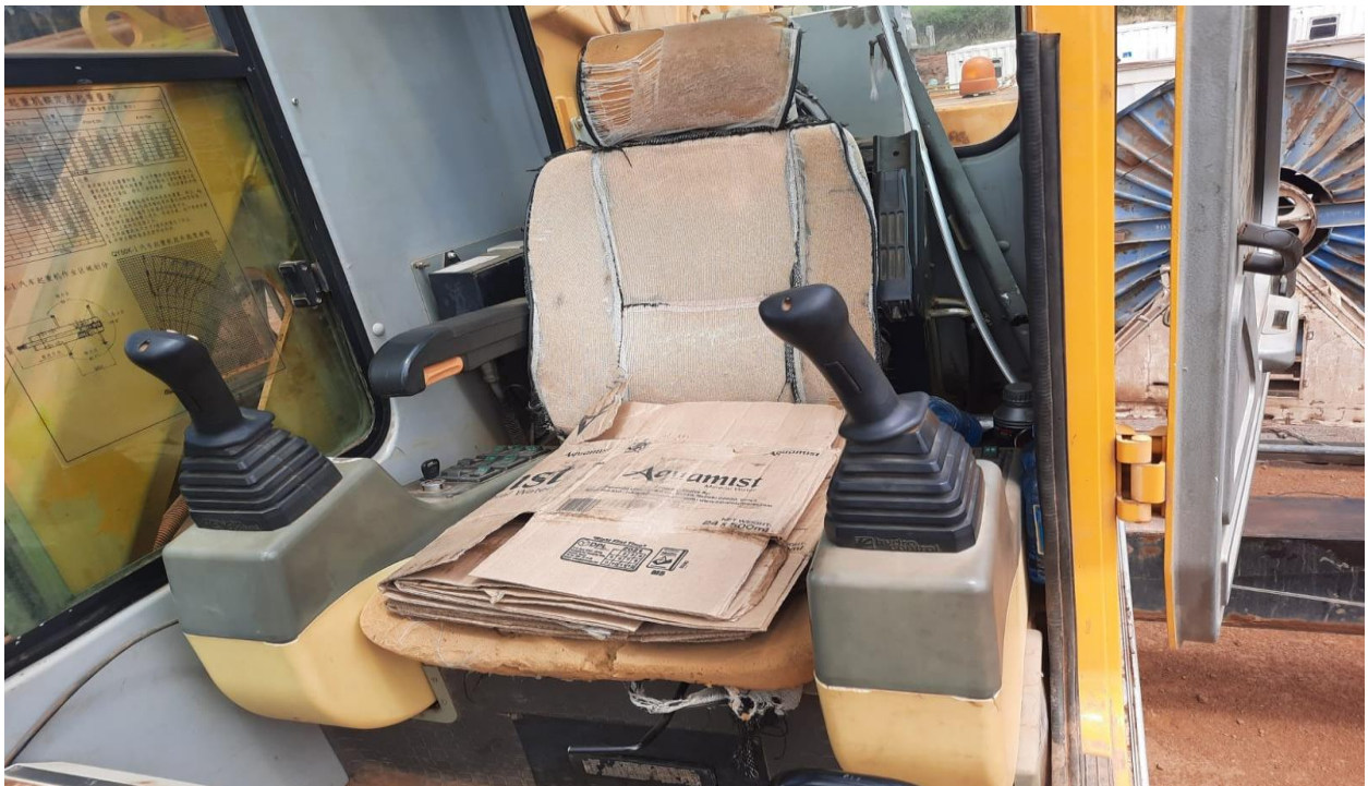
Plate 4. 7: Crane Operator Seat Placed with Cartons which is Uncomfortable
