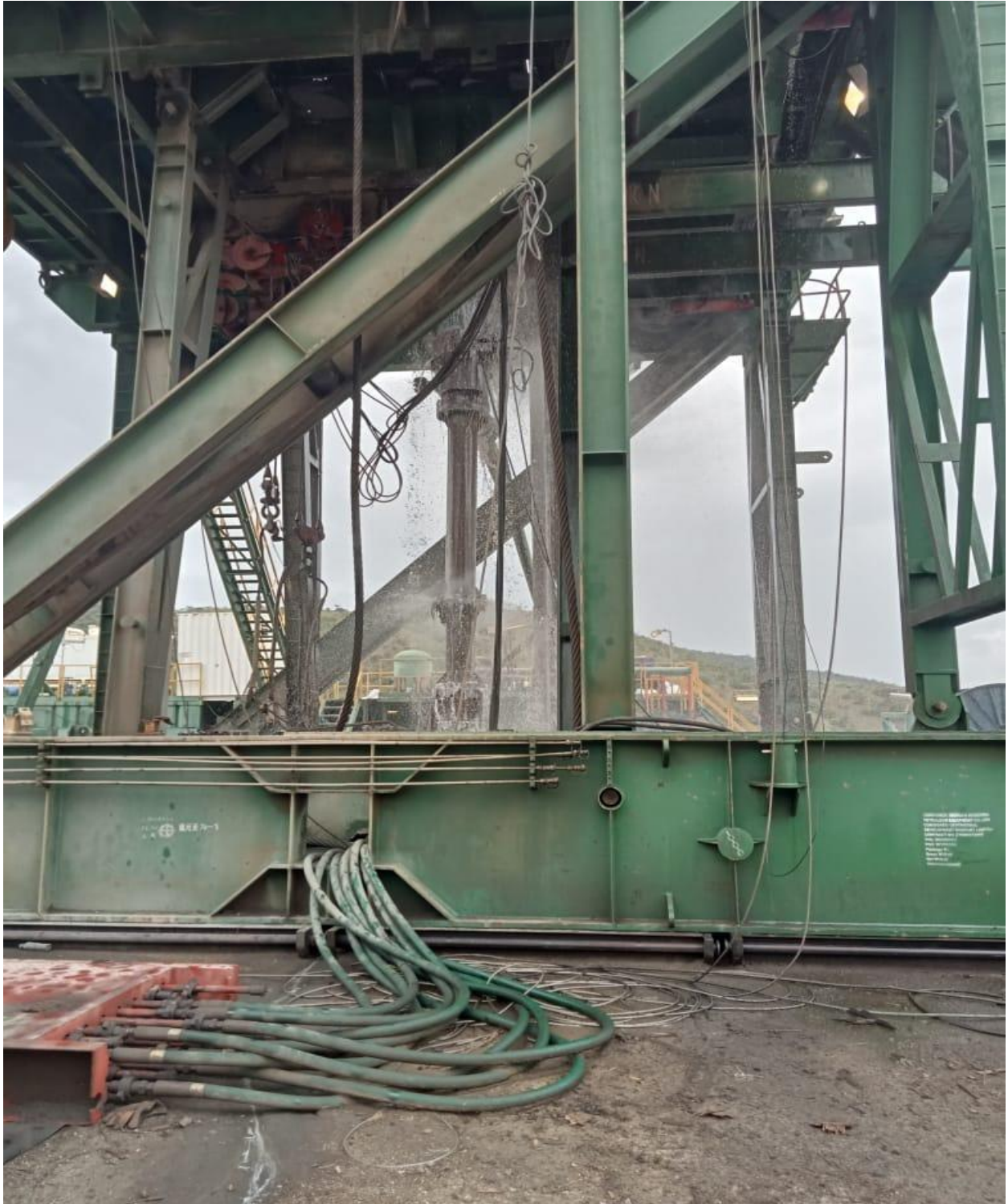
Plate 4. 4: Existence of Well Head Fluids
