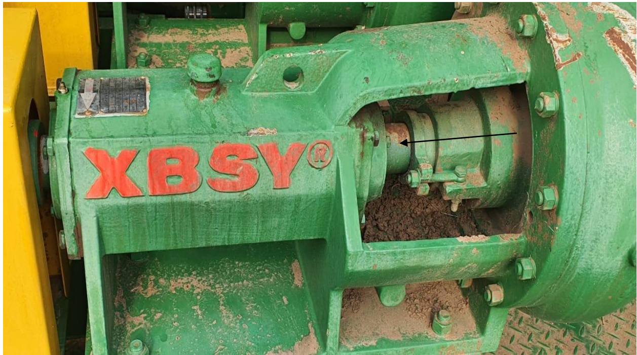
Plate 4. 10: Exposed Machine Propeller for Mud Mixing Motor
