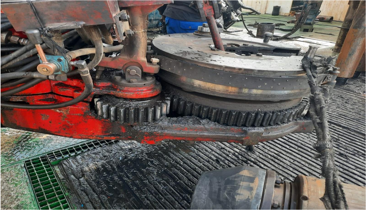
Plate 4. 8: Exposed Sharp Gears from a Power Tong Drillind Machine
