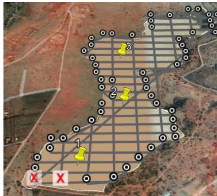
Figure 3.5: Bathymetric survey transects and ties lines orientation
