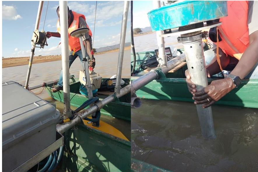
Figure 3.8: Sediment coring process
