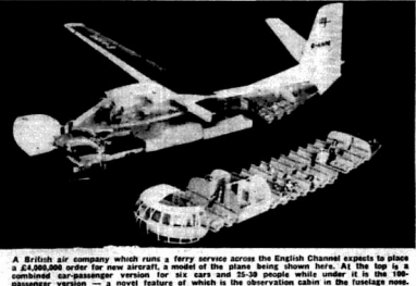
A British air company which runs a ferry service across the English Channel expects to place a £2,000,000 order for new aircraft, a model of the plane being shown here. At the top is a combined car-passenger version for six cars and 50-60 people while under it is the 100-passenger version — a novel feature of which is the observation cabin in the fuselage nose.
