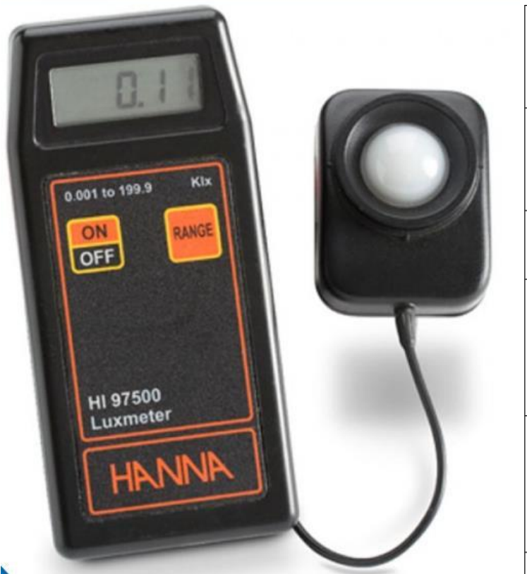
Appendix Figure 1 - 3: Luxmeter HI 97500 with specifications
