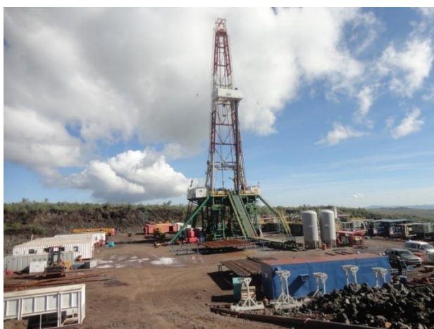
Figure 2 - 5: Conventional land rig as found in Menengai
