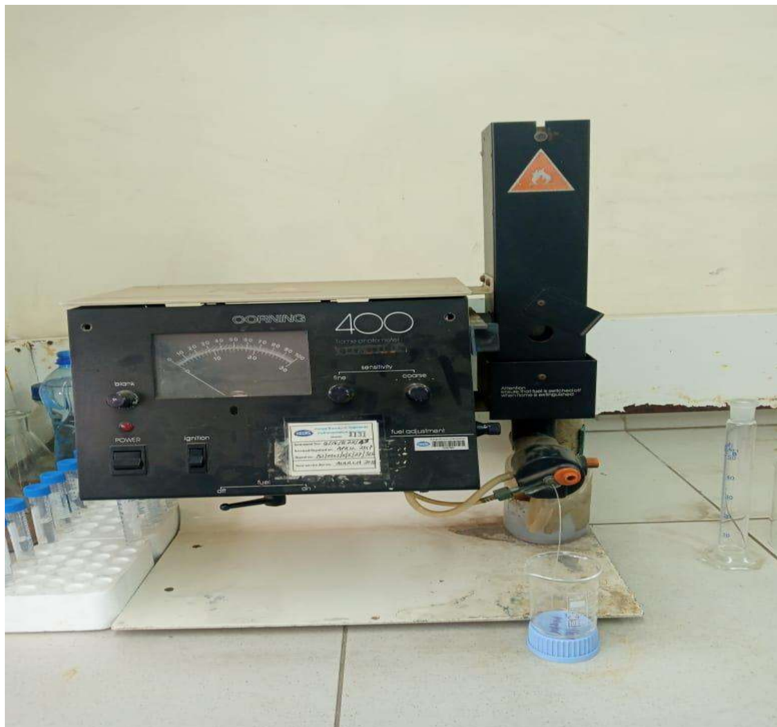
Figure 3.7: Corning 400 Flame Photometer, Kenya Bureau of Standards, Kenya
