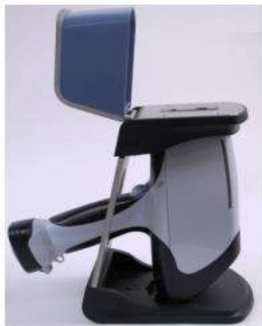
Figure 3.1: S1 Titan Bruker Model S1 Titan 600 series 600N 3187- MFG May 29, 2015, Mines and Geology Department, MOE, Kenya
