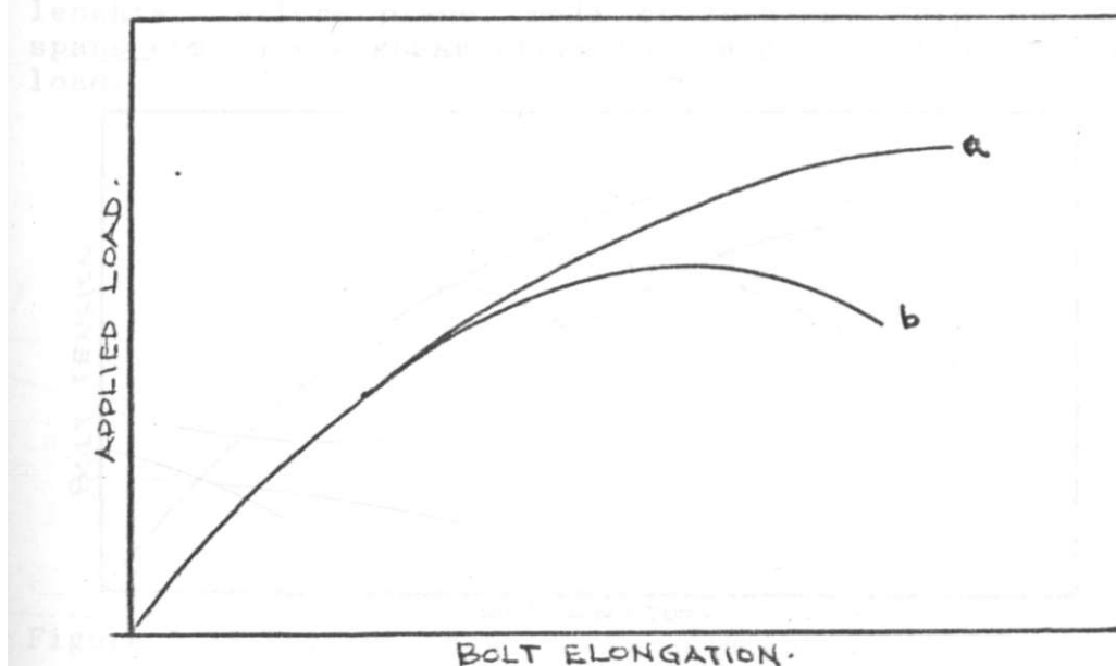
Figure 3.28 Load-elongation curves for bolts tested in:- (a) direct tension (b) torqued tension
