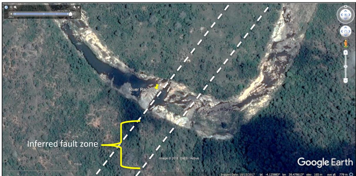
Figure 5-4 A natural colour satellite image (bands 4,3,2) of NE-SW trending knick points within a fault zone intersecting River Marere bed, north of Kwale town. (©2019 Used with permission from Google LLC. Google LLC's registered trademarks include Google and the Google logo.)
