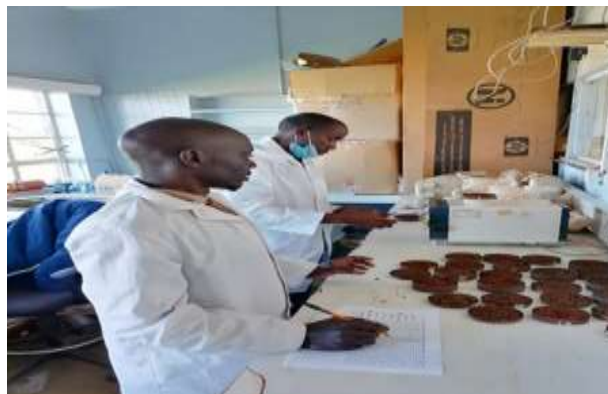
Plate 4.6: Determining moisture content from the sample soil in the Laboratory at TRI
