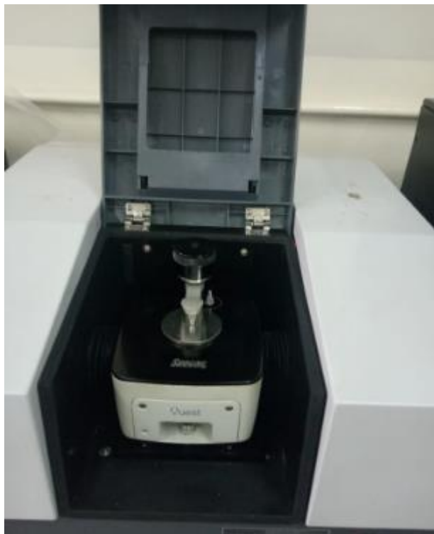
Figure 12: Fourier Transform Infrared spectrometer
