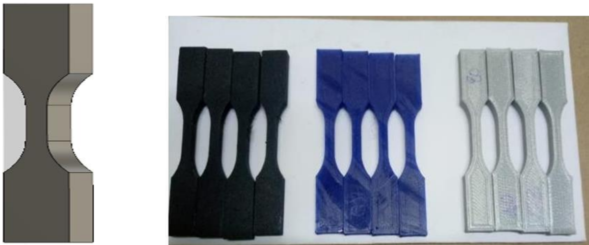
Figure 14a: Polymeric tensile test specimens
