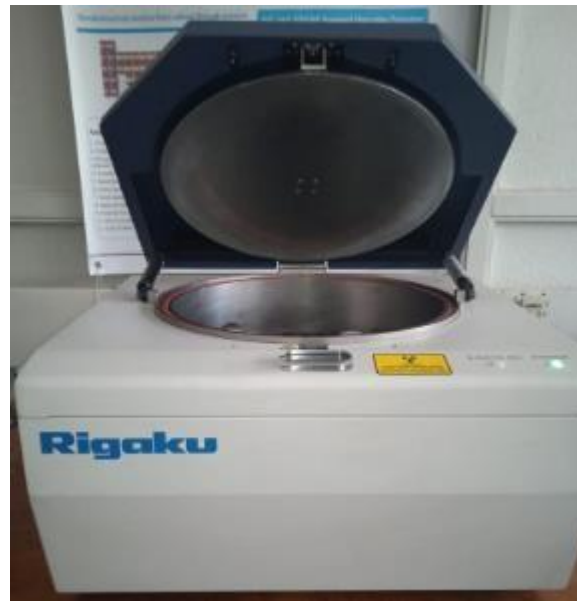
Figure 13: Energy dispersive Xray fluorescence spectrometer
