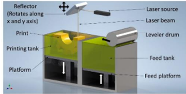
Figure 5: Selective laser sintering machine working based on the 3-D powder binding technology principle (Nath & Nilufar, 2020).
