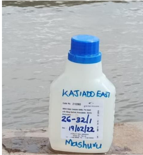
Figure 3.3: A 250 ml-water sample collected from cattle’s water trough in Mashuru sub-county, Kajiado County
