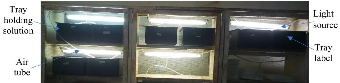
Figure 3.1: Screening chamber installed with trays holding screening solution, light source and air tubes supplied by an electric air pump.
