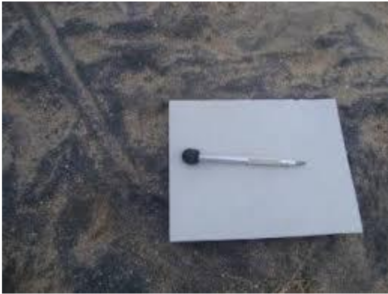
Fig. A.1 A pen magnet used to attract the black sands along the river channel.
