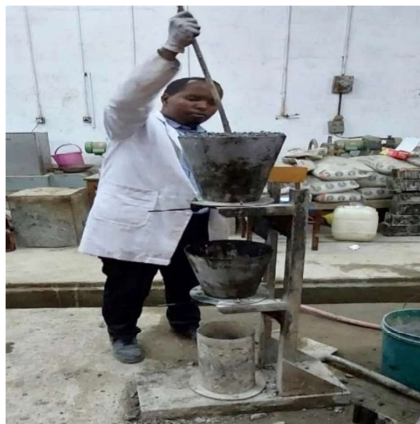
Figure 3.12: Compaction factor test of GPC
