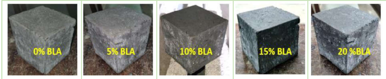
Figure 4.18 (c) Appearance after 56 days of immersing in a 5% NaCl solution
