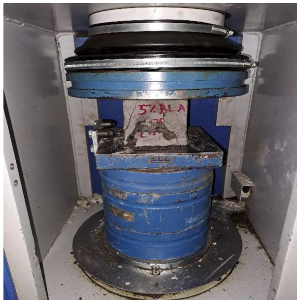
Figure 3.14: Compressive strength test
