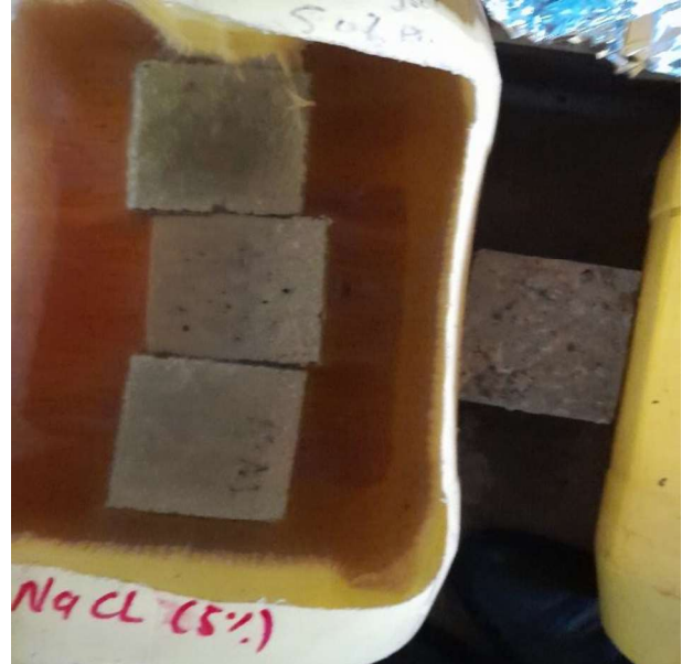
Figure 3.17: After the specimens immersed in the 5% NaCl solution
