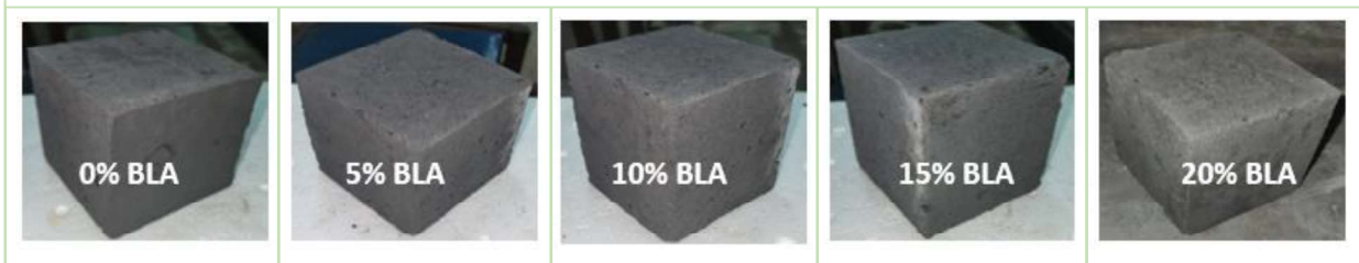
Figure 4.15 (d) Appearance after 90 days of immersing in a 5% H 2 SO 4 solution
