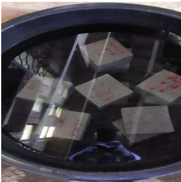
Figure 3.18: After the specimens immersed in the 5% MgSO 4 solution
