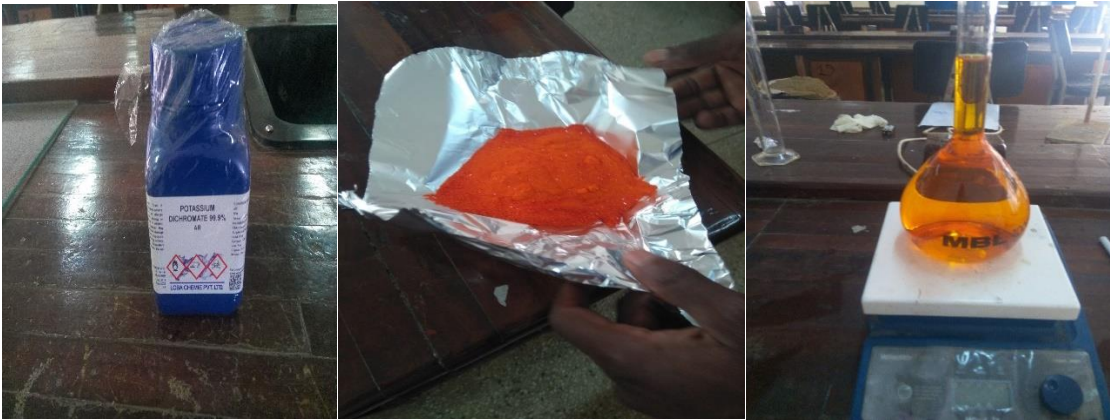
Plate 3.3: Potassium dichromate used for contamination
