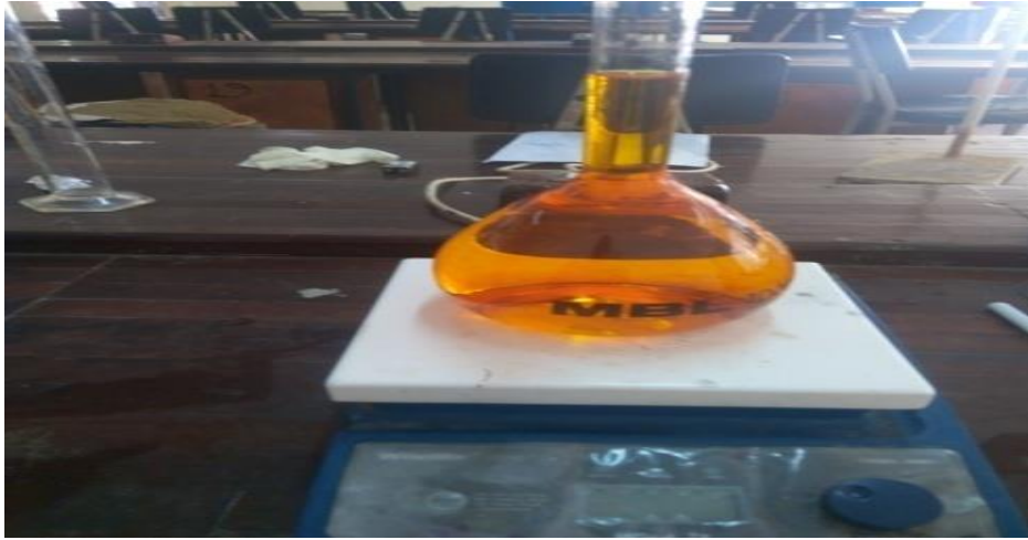
Plate 3.2: Potassium Dichromate mixture used to contaminate the red soil.
