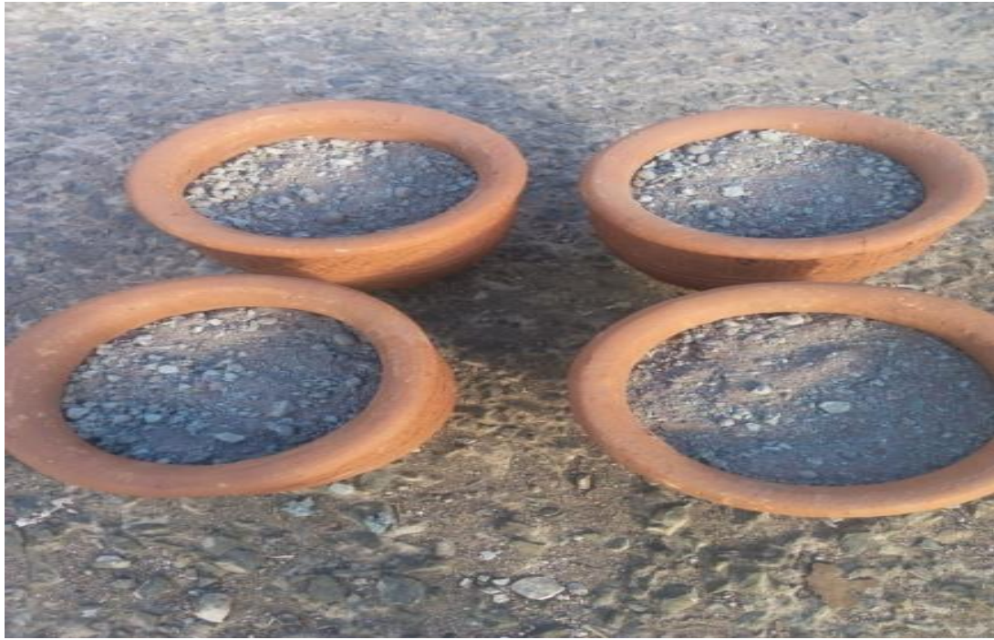
Plate 3.3: Pots containing mixture of tannery sludge and red soil
