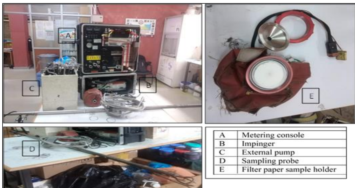
Figure 2-5: Typical isokinetic source sampling train (Source: author)
