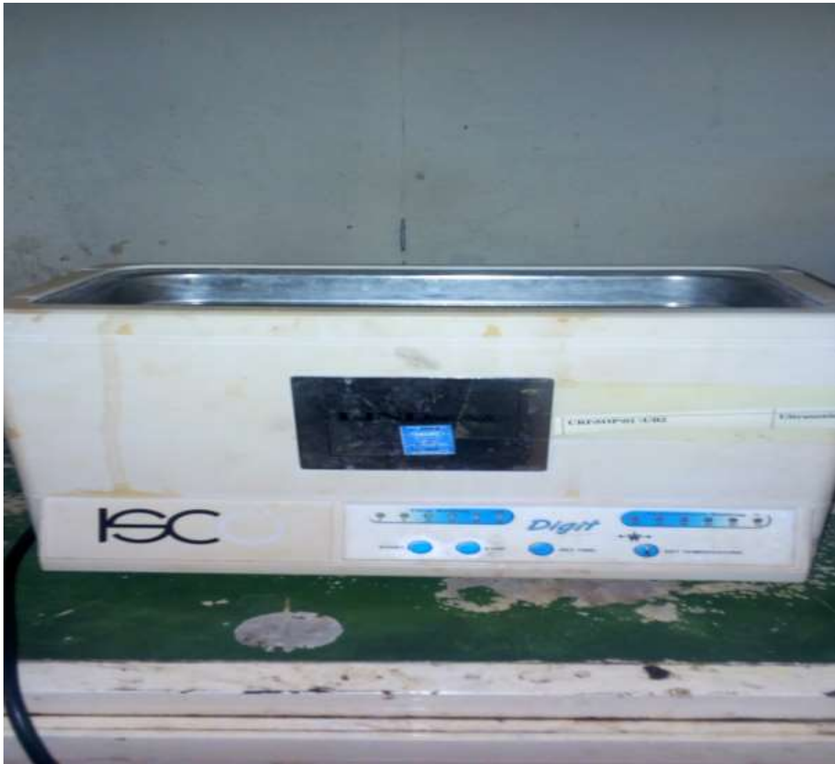
Diagram 7.4: ultrasonic bath for homogenization used during analysis
