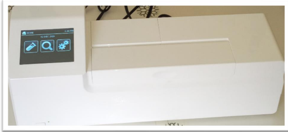
Figure 4-2: The Axxin T8-ISO instrument used for isothermal amplification.
