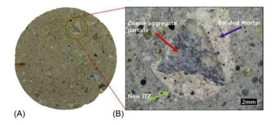
**Figure 1:** (A) Mortar adhered on coarse aggregate, (B) magnification of adhered mortar on coarse aggregate showing bonded mortar, coarse aggregate particle, and interfacial transition zones (ITZ) **Source:**(De Brito & Saikia, 2013)
