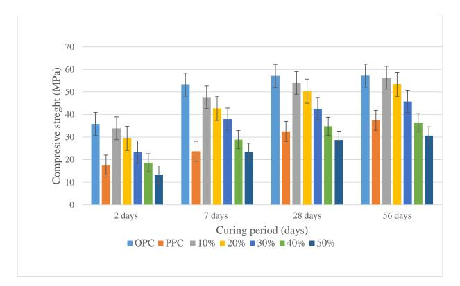
Figure 4: A graph of compressive strength against curig period
