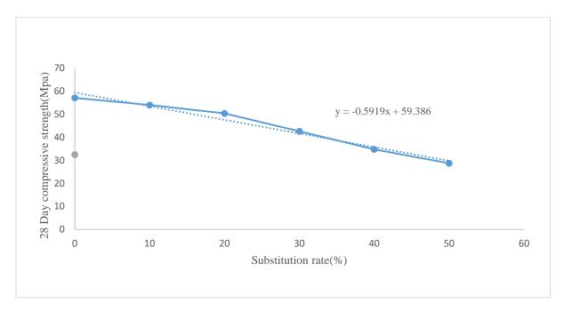
Figure 7: A graph of 28-day compressive strength against substitution rate.
