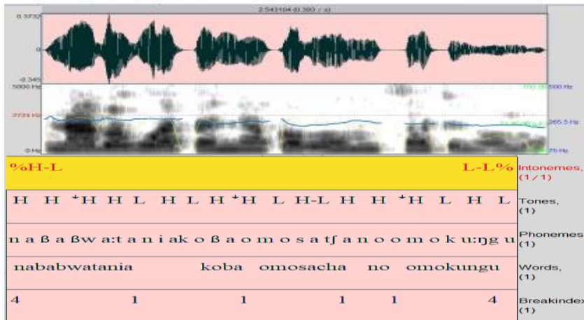
Figure 3.7: Audio waveform, F0 contour and ToBI label window for /náβáβwá:tániá kòβá ómòsâtfá nó ómòkú:ngú/ produced by a 9-year old female
