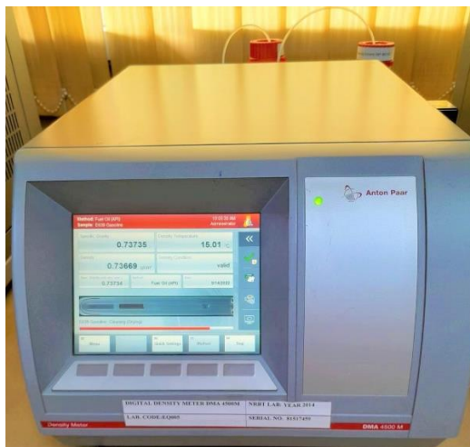
Figure 3.2: A Digital Density Meter
