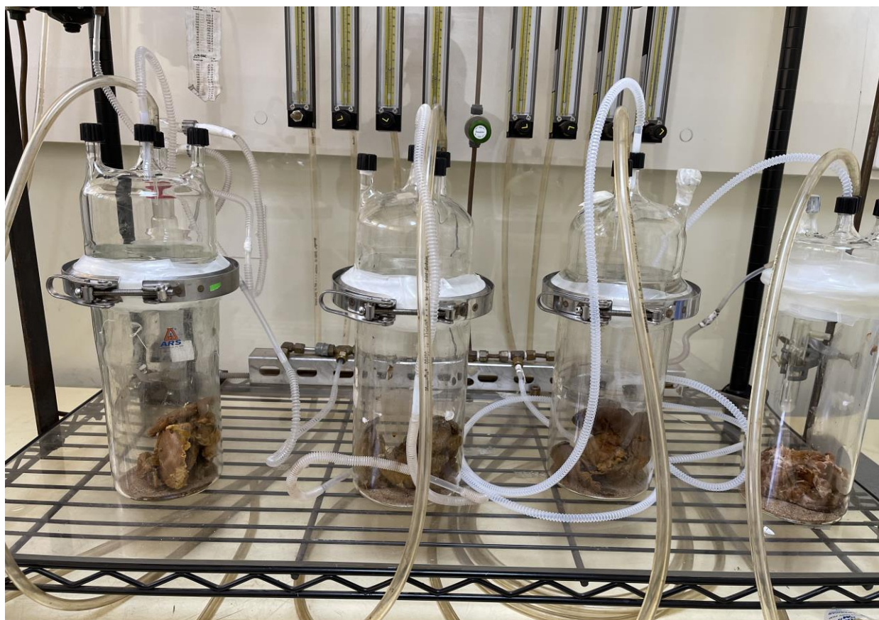
Figure: 3.0. Image of the air-tight trapping jars for headspace trapping of the chemical volatiles at icipe chemistry laboratory
