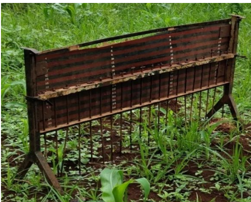
Plates 3.2a (left) and 3.2b (right): Relief meter and a handheld penetrometer
