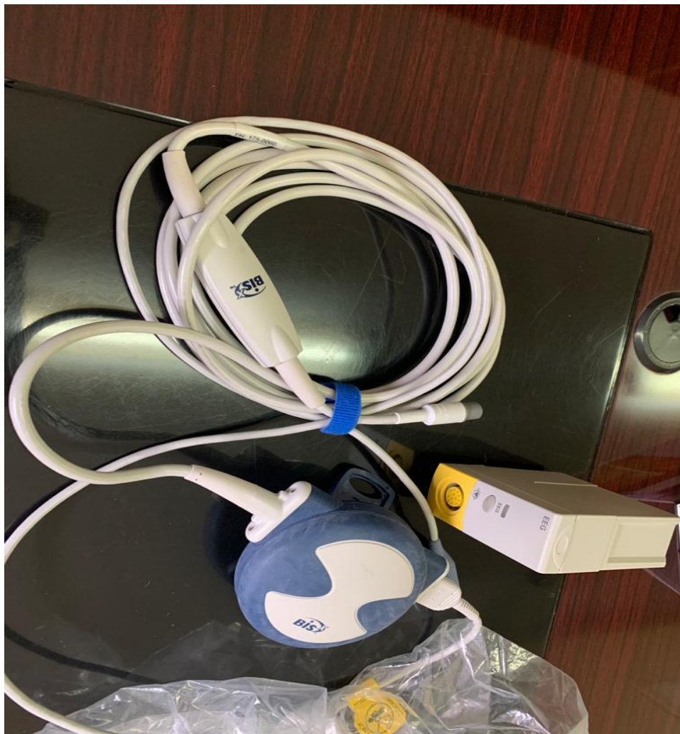
Figure 10: An image showing a Philips™ BIS Monitoring Module
