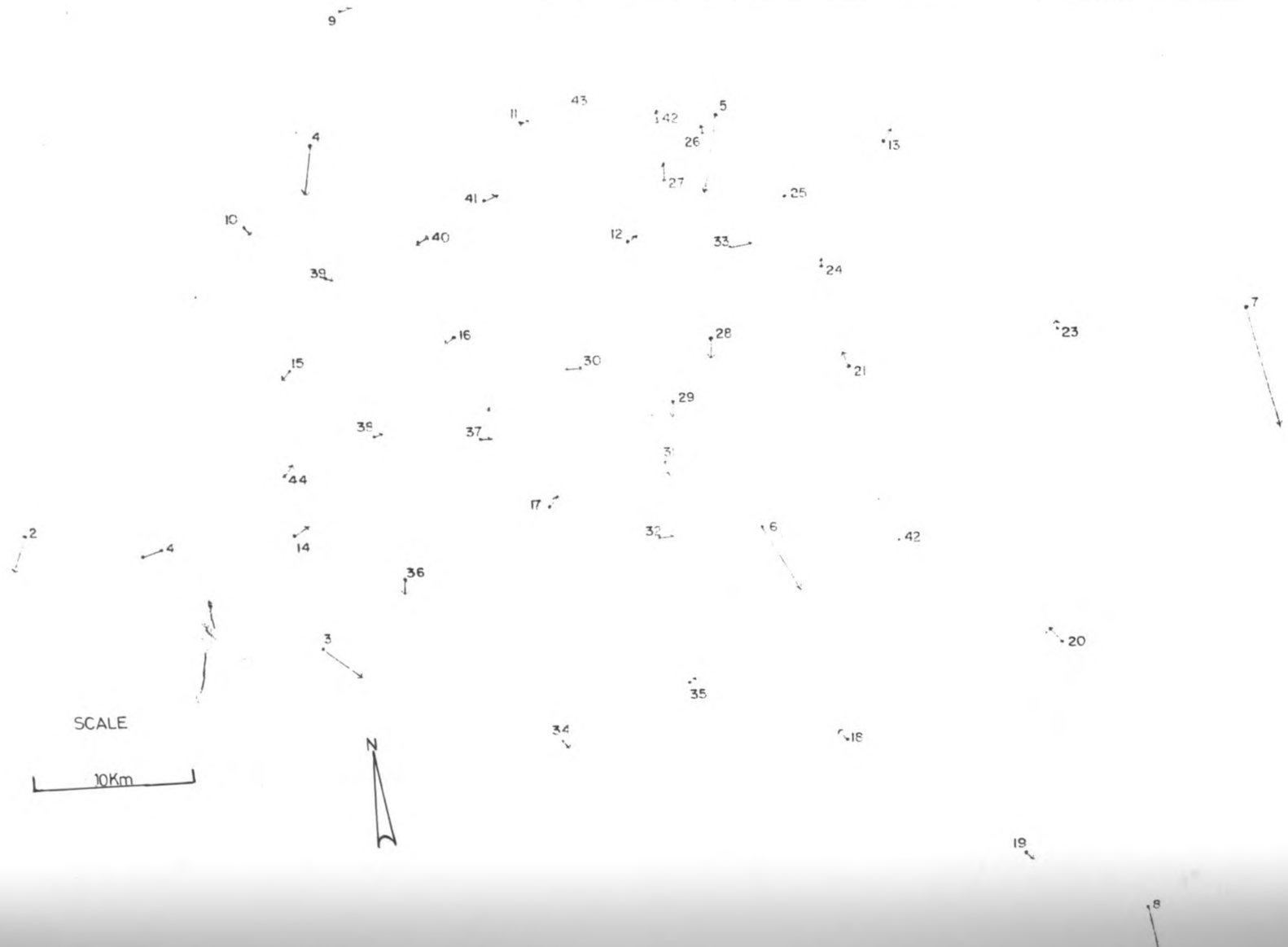
FIG 13 EXPERIMENT C SHIFTS OF POINTS FROM THEIR POSITIONS AFTER TO THEIR POSITIONS AS A RESULT OF STATIC-DYNAMIC DENSIFICATION.
