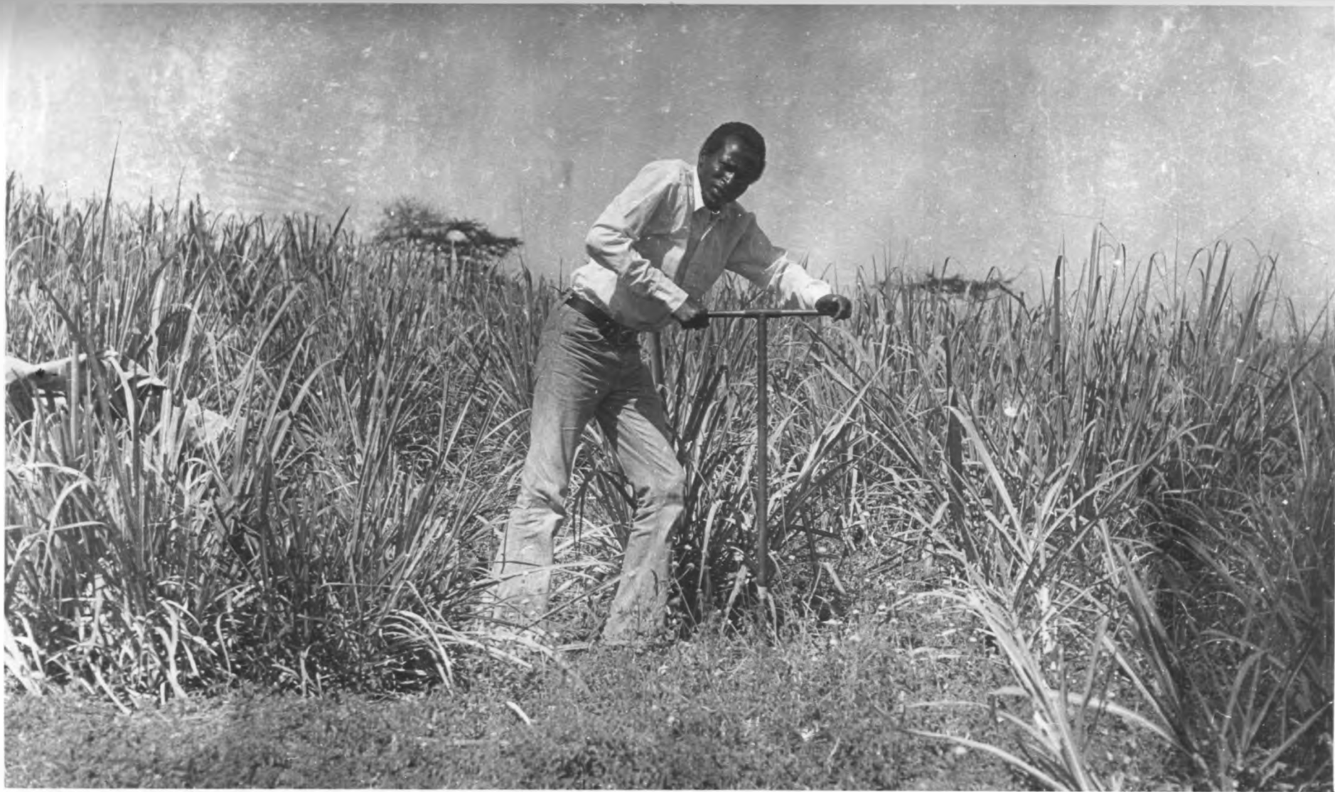
Fig. 4. Composite Soil Sampling in sugarcane cultivated plot on farm by the author. The White mark on the auger indicates 0-30 cms. drilling limitation
