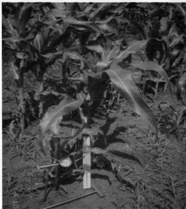
Plate 3. Placement of tensiometer in sweet corn rows. Note the T-bar auger for making the holes.
