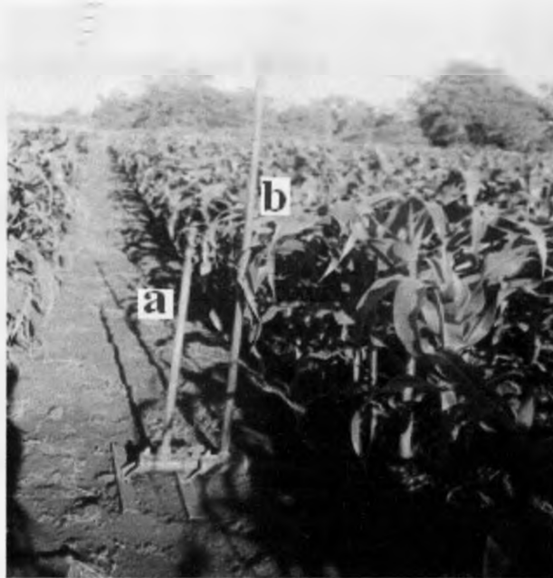
Plate 2. Two types of sprinklers used for irrigating sweet corn; a - single riser and b - double riser.
