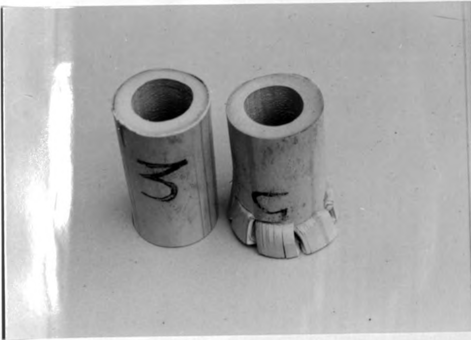
Fig. 5.3: Failure in Compression (Without Nodes)
