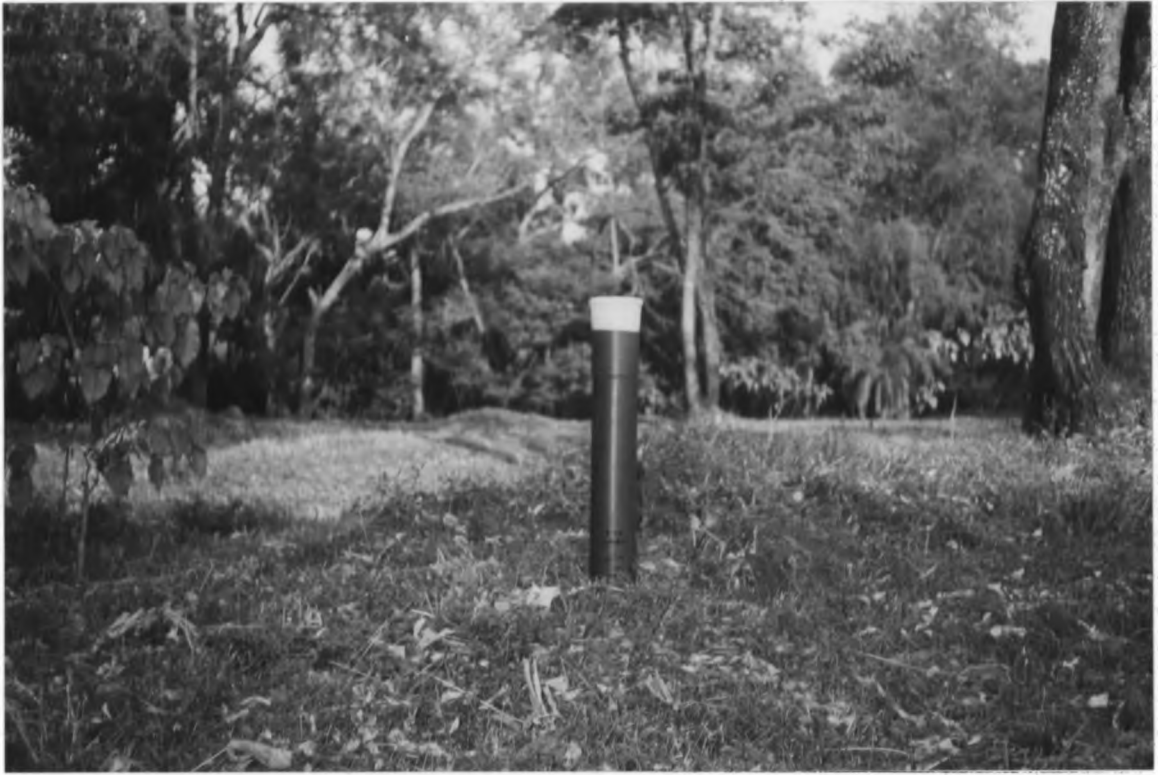
PLATE A: A termite trap (a PVC pipe sealed at one end) inverted at the mouth of a termite nest.
