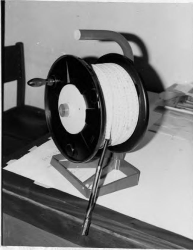
Plate II Electric Dipper used for Water Level Measurements
